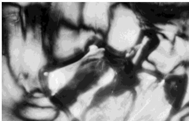
Figure 1. Transient birefringence (reminiscent of nematic threaded textures) observed by optical microscopy under polarized light (polarizers crossed) from a sheared concentrated gel of \text{KPdPS}_4 in DMF.
